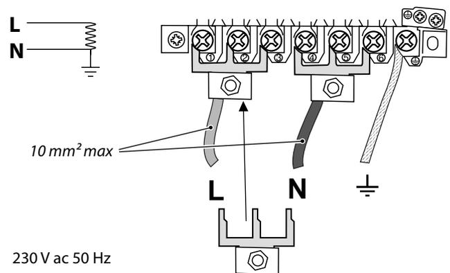
Access to the mains terminal is gained by removing the electrical terminal cover box on the back panel. Connect the mains cable to the correct terminals for your electrical supply type. Check that the links are correctly fitted and that the terminal screws are tight. Secure the mains cable using the cable clamp.
