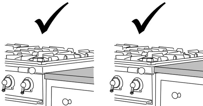
Adjacent work surfaces should be level with or below the hotplate surround – **NOT** the pan supports.
