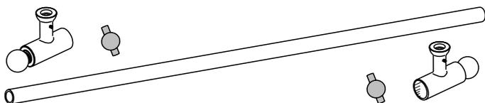
Hold a friction cup by the tabs on one end of the tube. Fit one of the end pieces to the tube and push it on the tube over the friction cup.
