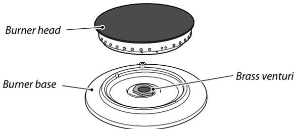
When fitting the burner head, make sure it locates properly within the burner base.
