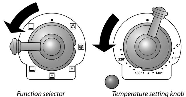
Turn the function selector control to a cooking function. This is the fan oven setting.
