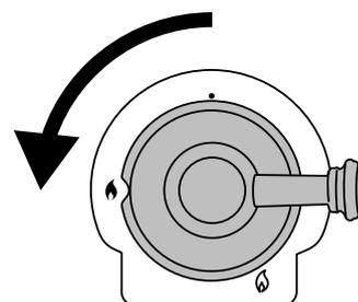
Keep holding the knob pressed in to let the gas through to the burner for few seconds. The igniter should spark and light the gas.
