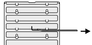
Lift up the front of the shelf so the back of the shelf will pass under the shelf stop and then pull the shelf forward.
