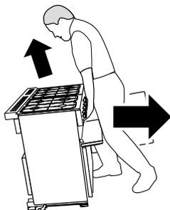
Carefully push the cooker backwards off the base tray. Remove the base tray. Position the cooker close to its final position, leaving just enough space to get behind it.
