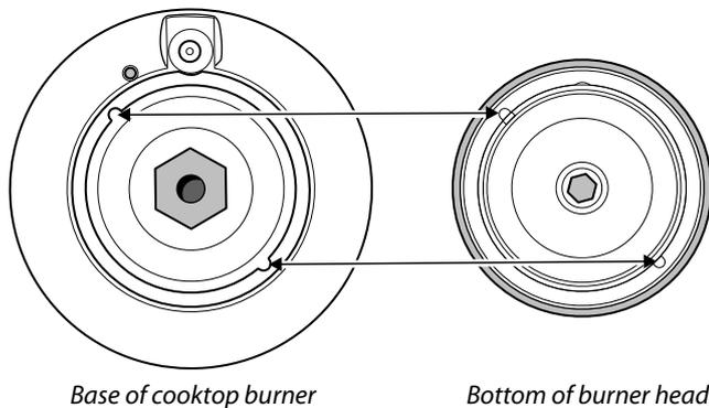
If you look at the bottom of the burner head you will see two 'pips'; these fit into the two notches in the burner base.
