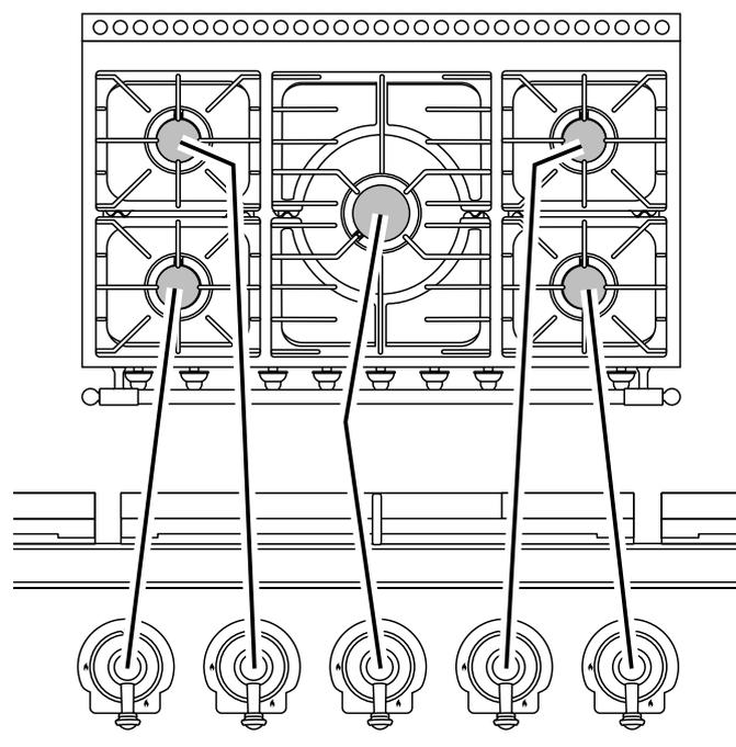
There is a spark ignition system that works when the knob is pressed in. Each burner also has a special safety device that stops the flow of gas if the flame goes out.
