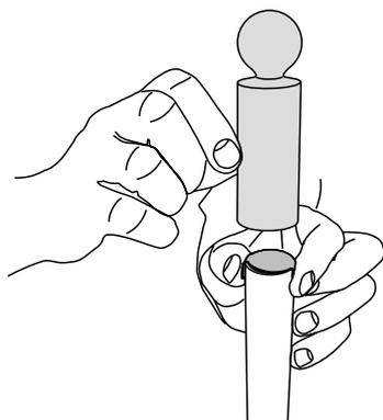
Turn the tube over and fit the other end piece using the second friction cup, making sure that you do not scratch or damage the first end piece and that the two end pieces are lined up correctly.
