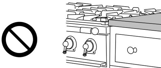
We recommend a gap of 900 mm between units to allow for moving the cooker. If a flush fit is required, fit the cooker up
