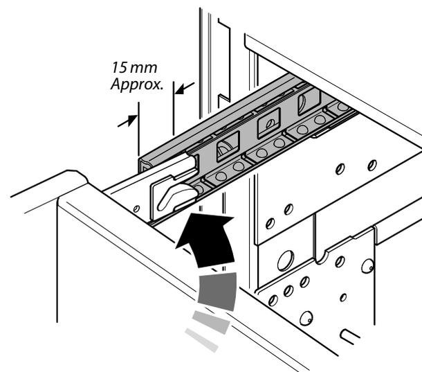
Rotate the drawer to locate the remaining drawer rail onto the opposite inner side rail.
