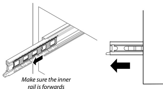
Lift the drawer at its sides and locate one of the drawer rails (approximately 15 mm) onto an inner side rail.
