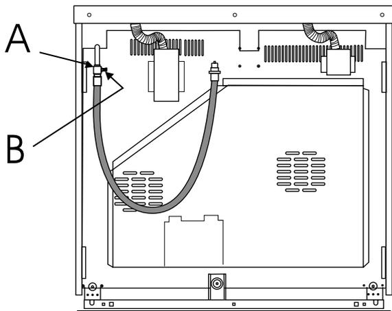
Because the height of the cooker can be adjusted and each connection is different it is difficult to give precise dimensions. The hose should be fitted so that both inlet and outlet connections are vertical so that the hose hangs downwards in a 'U' shape.
